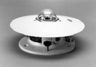
desiccator that can be readily inspected. The instrument has a cast bronze body with a white enameled guard disk (shield).
