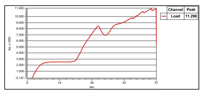
Manu. Min. Break Load (NBL) lbs: 11600 Test Results (Max Load) lbs.: Broke at termination
