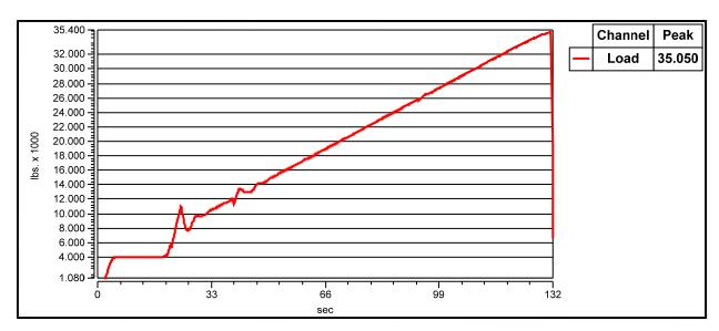
Manu. Min. Break Load (NBL) lbs: 32500 Test Results (Max Load) lbs.: Broke at termination
